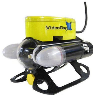
Figure 2. VideoRay ROV used to conduct the benthic composition survey.
