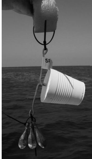
Figure 3. This image shows the final product just prior to deployment. This clod card design inverts the cards in the water column.
