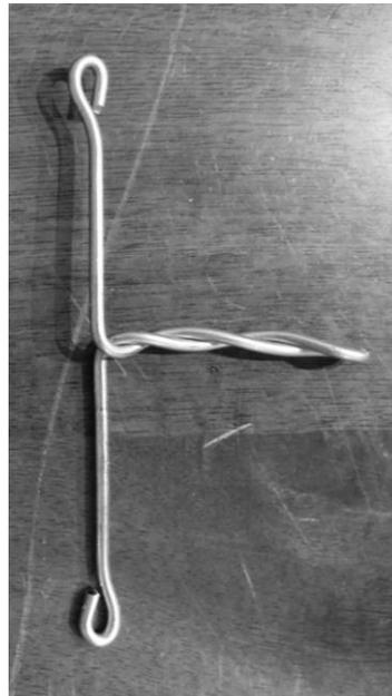
Figure 2. This image shows the “T” shape made from galvanized steel wire.
