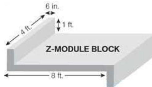
Figure 1: Illustration of the standard dimensions and shape of the artificial reef Z modules used at the Waianae Artificial Reefs
